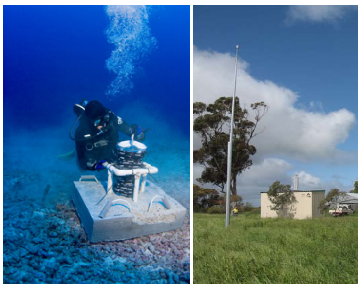
(left) Acoustic doppler current profiler used to measure wave and current patterns, (right) weather station at Wilgerup Project near Lock.
