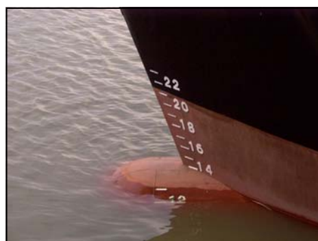
(left) Graph showing cost savings by using larger vessels, (above) Picture of drafts marks on vessel
